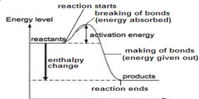
Reactions occur because of collision of particles and sufficient kinetic energy is needed to provide activation energy to break the bonds and start the reaction by providing extra energy from a heat source.
