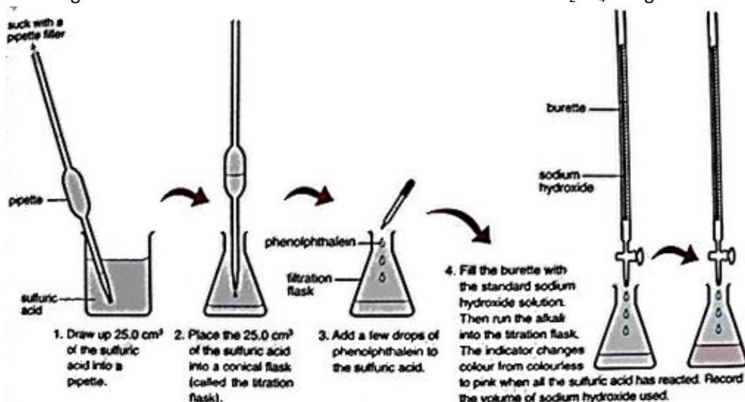
Using above example, to find the concentration of H<sub>2</sub>SO<sub>4</sub> is given on the next page
