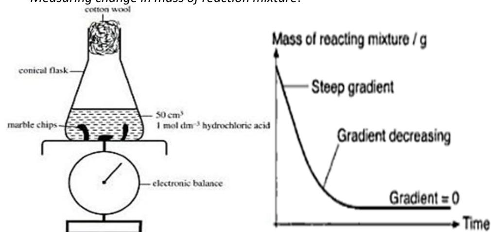
Marble is reacted with acid in a flask with cotton wool stucked at top to prevent splashing during reaction but it allows gas to be free. The reading on balance is plotted on a graph on every time interval.
