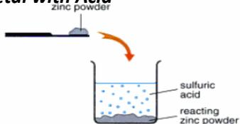
1. Add zinc powder bit by bit with stirring to hot dilute sulfuric acid until some of it no longer reacts. The acid is then used up. There is excess zinc present.
