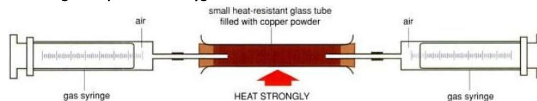
A known volume of air is passed through tube with burning copper powder and oxygen in air will react with hot copper powder to produce black copper oxide:
