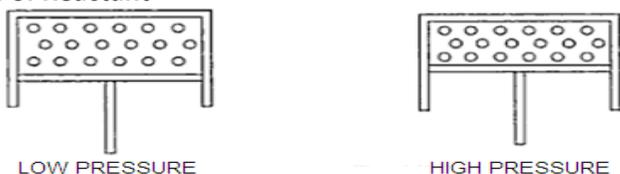
Only gaseous reactions are affected as gas is compressible. At higher pressure, molecules are forced to move closely together, hence increasing the particles per unit volume of gas and effectively increases the collision between reacting molecules so the speed of reaction increases.
