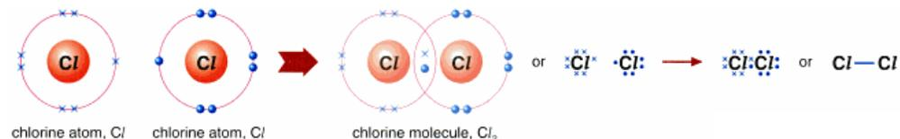
Cl atom has 7 valency and needs one electron, each, to form a noble gas configuration between two Cl atoms. Hence they share an electron EACH to hence share 2 electrons between the atoms. Hence, each Cl atom now has 8 valency which is a noble gas configuration.
