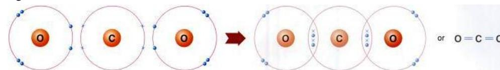
Carbon needs 4, oxygen needs 2. We share two from oxygen part, WHICH HAS THE SMALLEST NUMBER OF SHORT ELECTRONS, TO SHARE THE AMOUNT OF ELECTRONS THAT ATOM NEEDS, to form 4 shared atoms. Now oxygen is stable but carbon needs 2 more, which we now know they can get from another oxygen atom. The atoms are now stable and since each bond has 2 pairs of electrons, we call this double bond: C = O.
