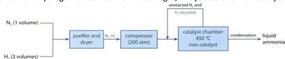
Since the reaction is reversible so  $\text{H}_2$  and  $\text{O}_2$ , reproduced from decomposition of produced  $\text{NH}_3$ , are passed over the catalyst again to produce ammonia.
