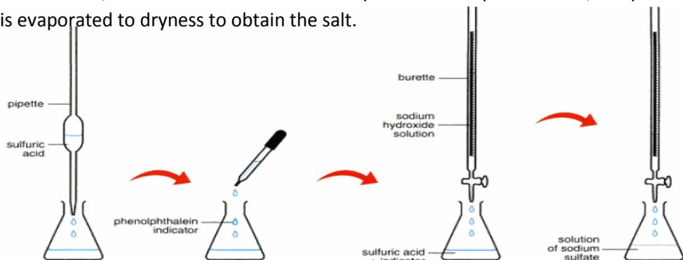
1. Using a pipette, 25.0 cm<sup>3</sup> of sulfuric acid is placed in a conical flask. A few drops of indicator are added (e.g. phenolphthalein).
