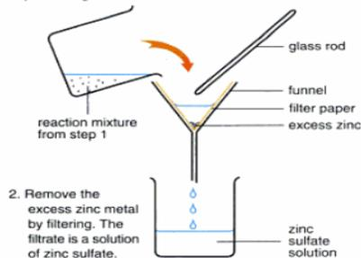
2. Remove the excess zinc metal by filtering. The filtrate is a solution of zinc sulfate.
