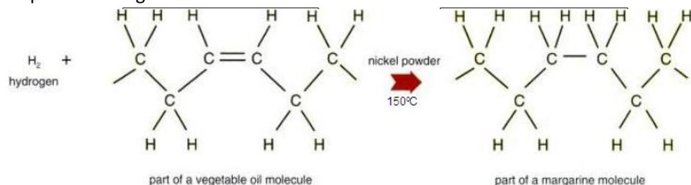
Hydrogen is reacted with vegetable oil with presence of nickel catalyst and heat, which adds to C=C bond, increasing the molecular mass of the compound
