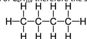
It has 4 carbon atoms bonded together with 10 hydrogen atoms
