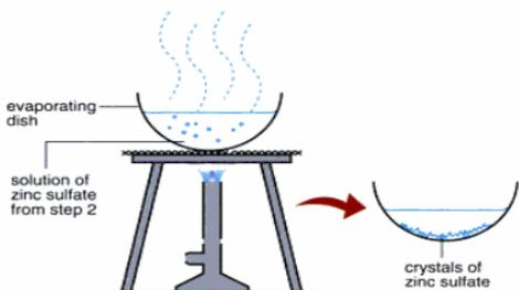
3. Pour the solution of zinc sulfate into an evaporating dish and heat to evaporate most of the water. This produces a hot saturated solution of zinc sulfate. Allow the solution to cool.
