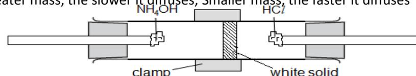
A cotton soaked in aqueous ammonia and another soaked in hydrochloric acid are placed on opposite sides of the tube. NH<sub>4</sub>OH vapor and HCl vapor diffuses in the tube and a compound is produced inside the tube closer to HCl soaked cotton as the particles are heavier. The greater mass, the slower particles diffuse. The smaller mass, the faster particles diffuse.
