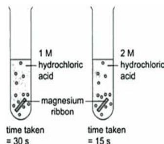
$$\text{Speed of reaction} = \frac{1}{\text{time taken}}$$
