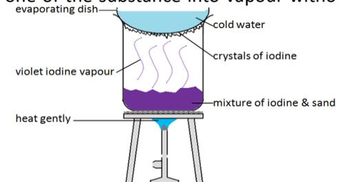
When mixture of iodine and sand is heated, iodine sublimates (turns into vapour directly) then cools and crystallise when it reaches cold water area
