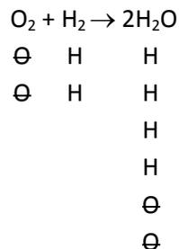
Now we can cancel off oxygen atoms. However, hydrogen atoms from reactant is short 2 atoms. Therefore, we multiply the hydrogen molecule by 2 so that the short is balanced. The equation is fully balanced when we are able to cancel off all atoms of that element on both sides.
