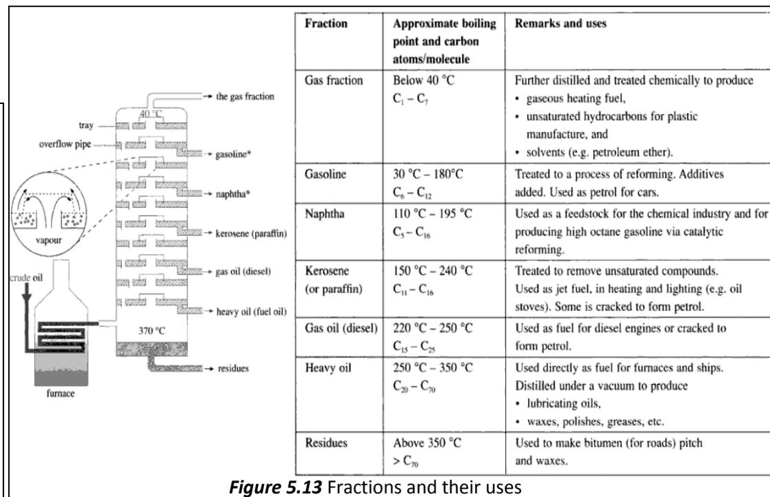
Figure 5.13 Fractions and their uses
