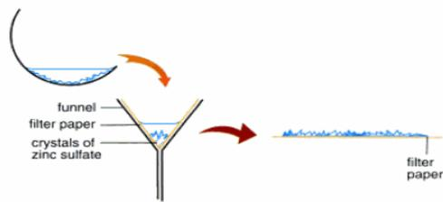
4. Filter the zinc sulfate crystals and dry them by squeezing them between sheets of filter paper.
