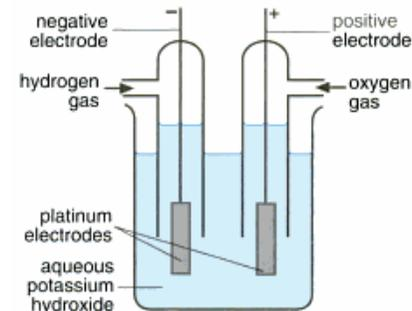
Hydrogen reacts with hydroxide ions into electrolyte on the platinum catalyst on electrode to make the electrode negatively-charged.
