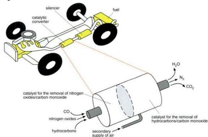
First, nitrogen oxides reacts with carbon monoxide as they pass a platinum catalyst.
