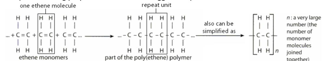
**Repeat unit** is the simplest part of the polymer which is repeated many times to form the polymer. We take the repeat unit to write the simplified formula of the polymer, where *n* is a large number. From this repeat unit, to find the monomer formula, we add double bond between C – C and remove the bonds on each of their sides.
