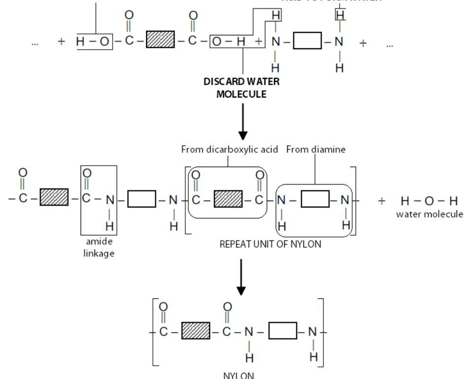
The linkage between monomers in nylon is called **amide linkage**. Therefore we can also call nylon as **polyamide**.
