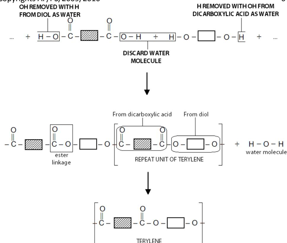
The linkage between the monomers in terylene is called **ester linkage**. Therefore we can call this polymer as **polyester**.
