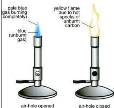
When air hole is closed, air cannot enter supplying oxygen, and hence soot (unburnt carbon) and CO is produced from incomplete hydrocarbon gas combustion. As a result, flame is yellow due to glowing specks of hot soot in heat and the flame is not hot. When air hole is opened, air supplies plenty of oxygen, allowing complete combustion.
