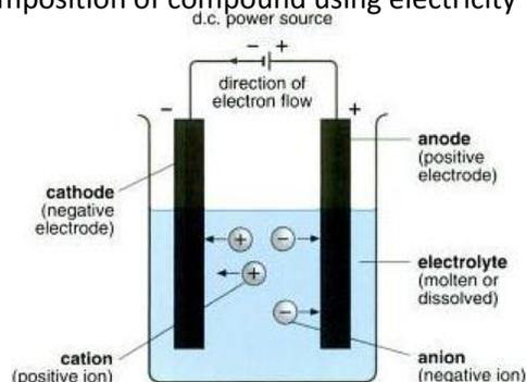
**Electrolyte** is an ionic compound which conducts electric current in molten or aqueous solution, being decomposed in the process.
