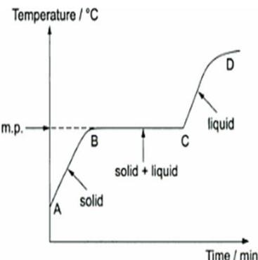
*Melting* is change from solid to liquid by absorbing heat to break force of attraction holding particles together. The temperature at which solid melts is *melting point*. From the graph:
